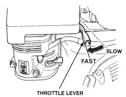
Figure 12. Throttle Lever
